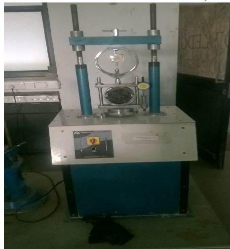
Fig 1 Marshall test apparatus with mould testing (Source –MEFGI highway laboratory)
