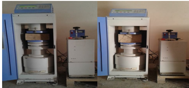
Fig. 4. Adobe blocks under compression
