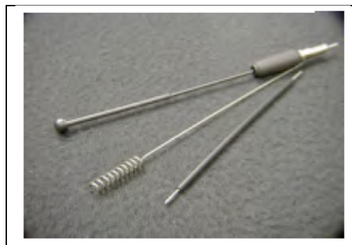
Fig 9. Photographs of cellular phone antenna.
