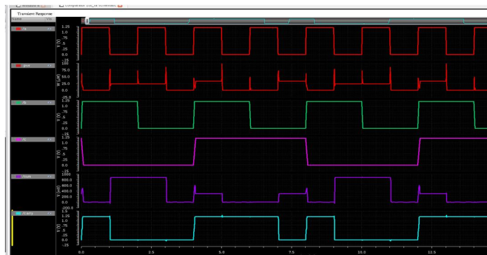
Fig.33. Output waveform for 45nm MUX 12T full adder
