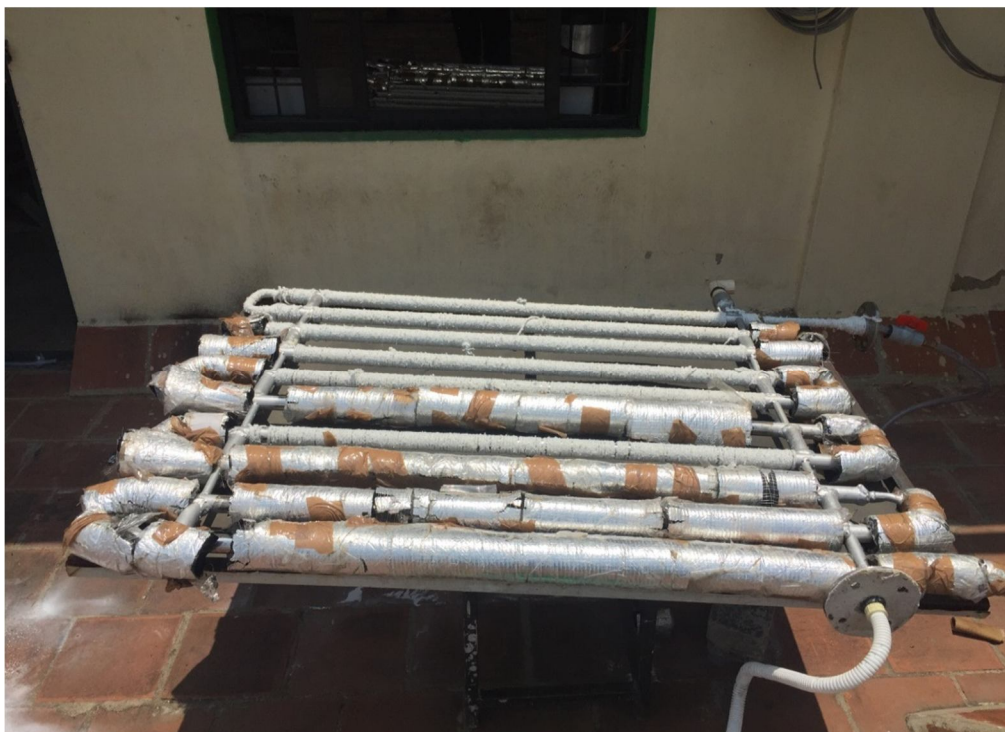
Fig 3.0 the above pipe in pipe heat exchanger is used for the experiment
