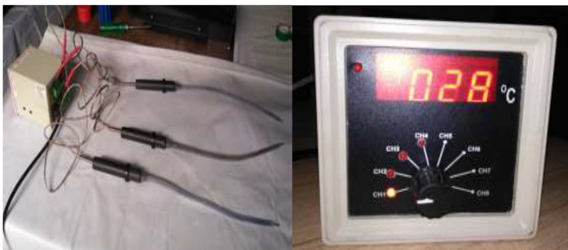
Figure 2 Thermocouples and temperature indicator
