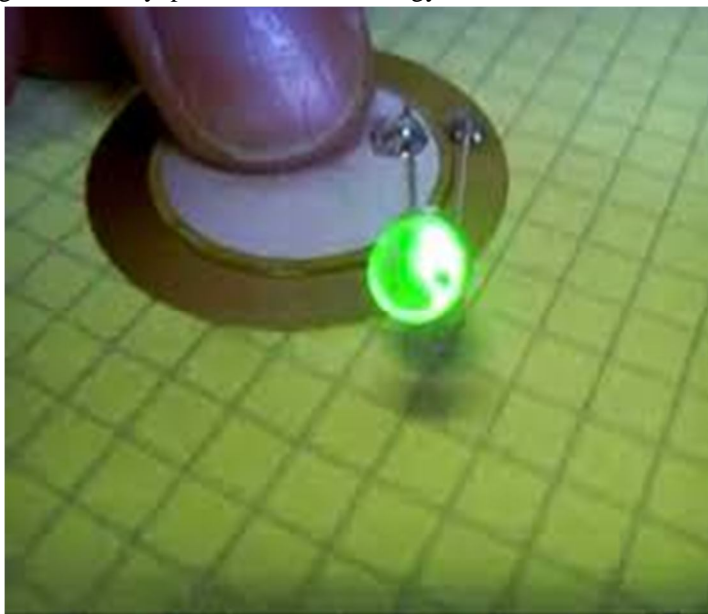
Fig: practical operation of piezo sensor with LED
