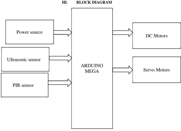
The above block diagram is the solar based automatic harvesting robot. The block diagram consisting ultrasonic sensor, PIR sensor and 12v power supply are act as the input signal, motors act as the output of the device.
