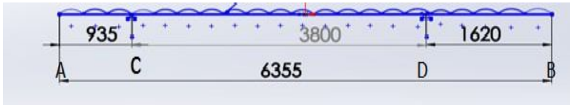
Fig.5. Load acting on chassis
