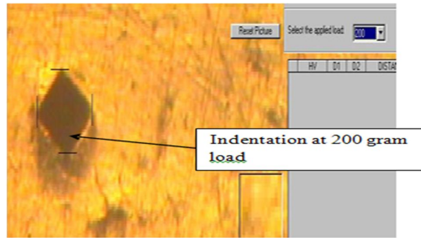
Fig. 4 – Micro indentation at 10X optical zoom
