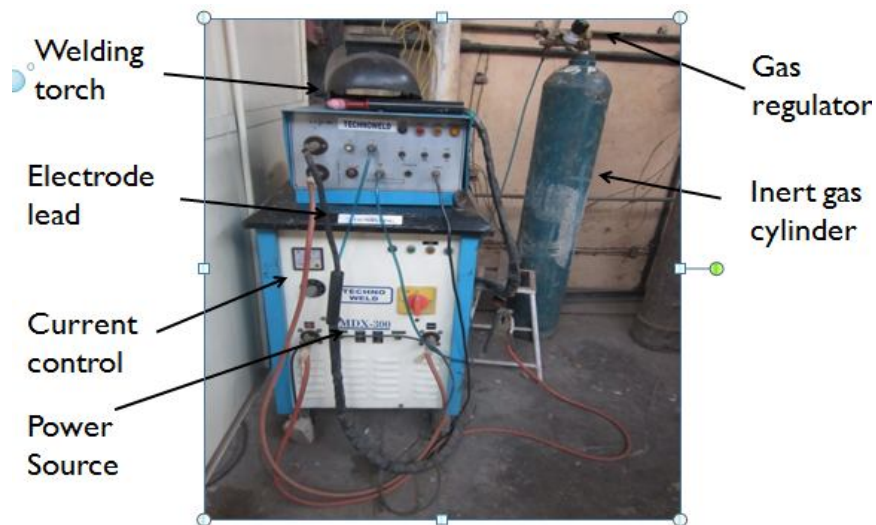
Figure 1: GTAW Setup (Courtesy: Paanchal Weld Workshop, Faridabad)
