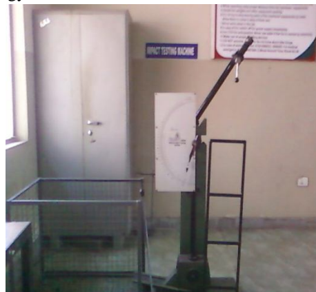
Figure 2: Impact testing machine (Courtesy: Solid Mechanics Lab, MED, MRCE, Faridabad)
