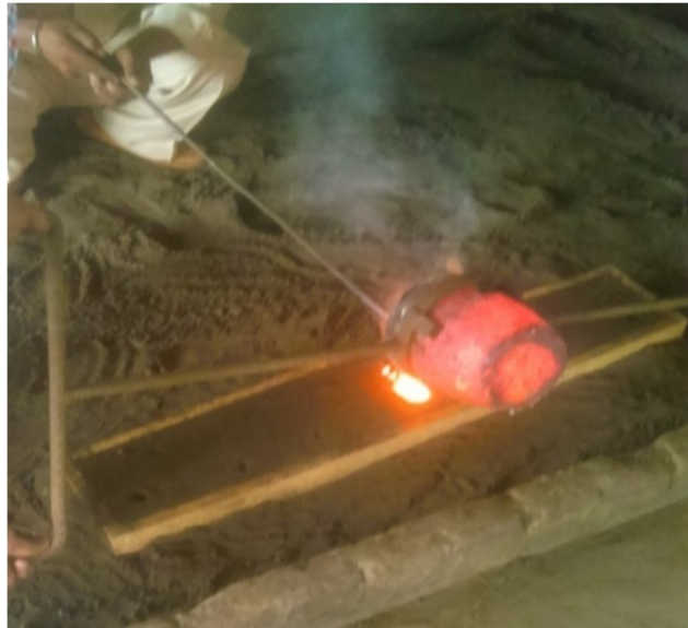
Fig. 1 Casting of MMC – Molten MMC being poured into mould
