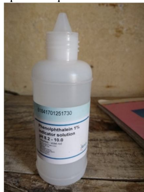
Figure 3 Phenolphthalein liquid used for carbonation test
