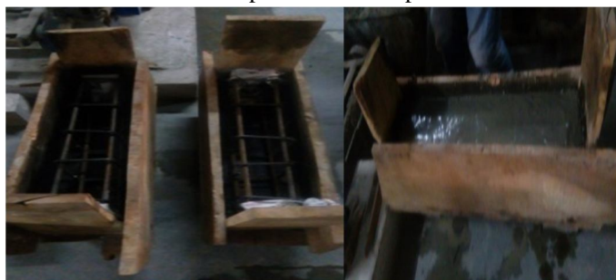
Fig.4 Moulds during casting.
