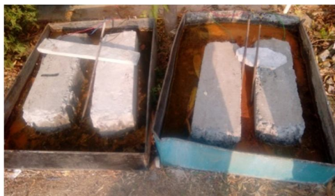
Fig.6 Accelerated corrosion process setup.
