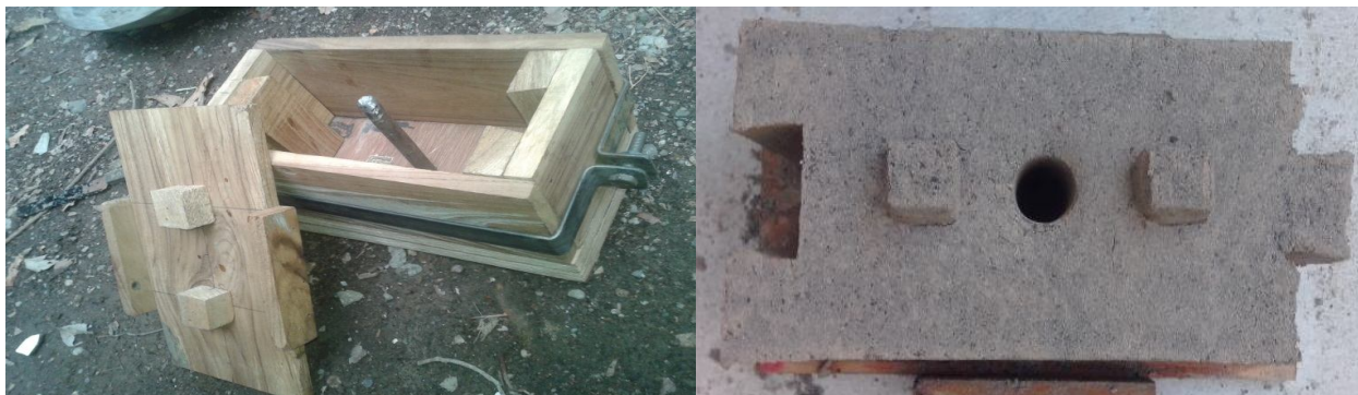
Fig 3: Mould and specimen ILB of model no. 3
