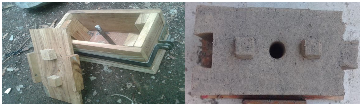
Fig 3: Mould and specimen ILB of model no. 3
