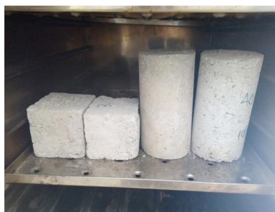
Figure 13: Lower Rate of Spalling in Plast-crete at Elevated Temperatures
