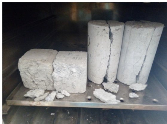
Figure 12: Higher Rate of Spalling in NC at Elevated Temperatures
