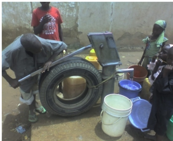
Plate1: Awkward posture of an operator on a lever type handPump
