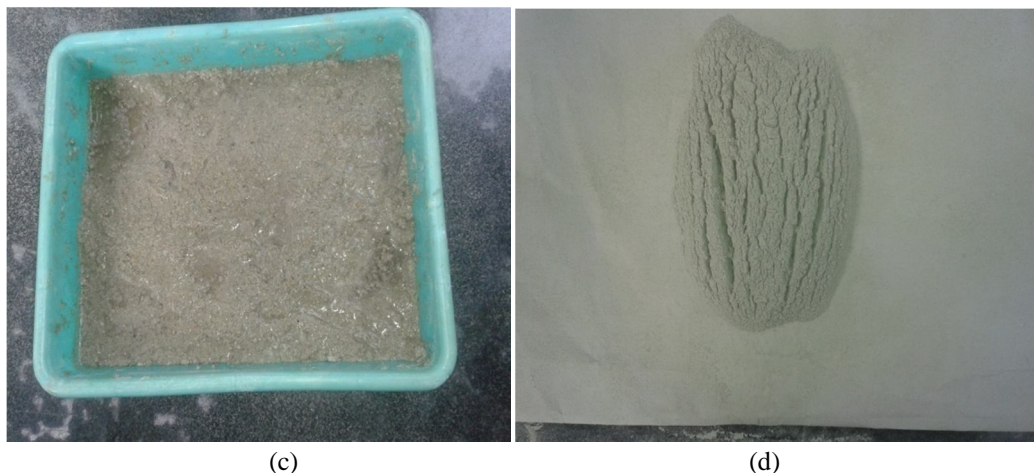
Figure 1: Collected samples (a) discarded PCBs before drying (b) discarded PCBs after drying (c) sludge before drying (d) sludge after drying in oven.
