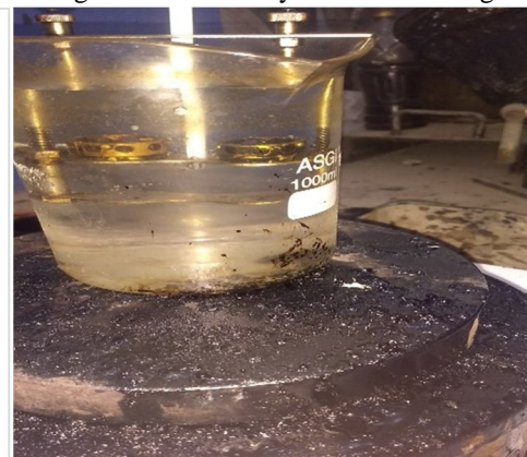
Fig. 6: Assembly for Softening point
