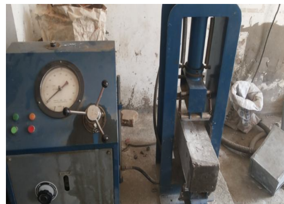
Fig. 6 Flexure strength test
