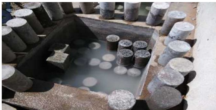
Fig. 11 Curing of specimen at specified days
