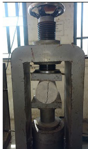
Fig. 12 Casting and Testing of Cylinder
