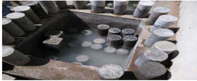
Fig. 13 Curing of specimen at specified days
