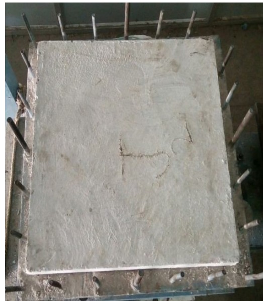
Figure 3: slab specimen placed on loading platform
