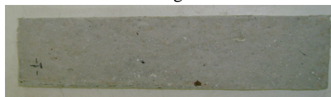
Fig. 4 Trimmed paper-based building specimen
