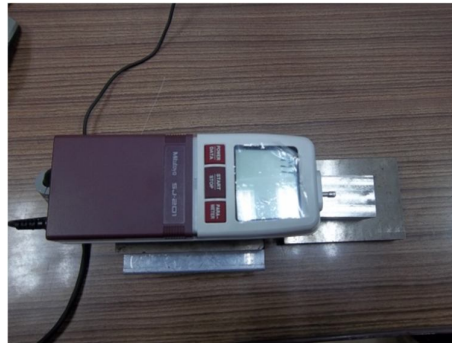
Fig 6.1 Measurement of Surface Roughness - Mitutoyo surf test SJ-200
