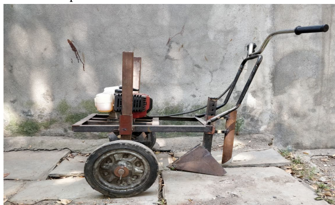
Fig. Basin Digging and Fertilization Machine
