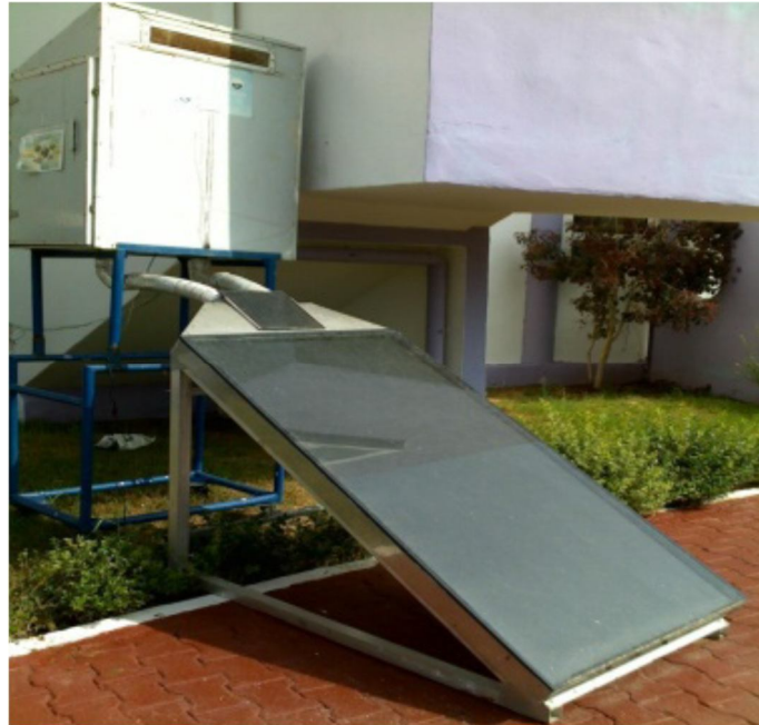
Figure 1: Schematic view of indirect solar dryer by Amina Benhamou et al. [7].
