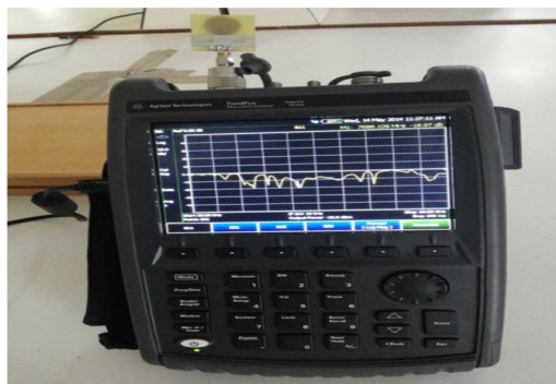
Fig.21.Fabricated antenna with network analyzer
