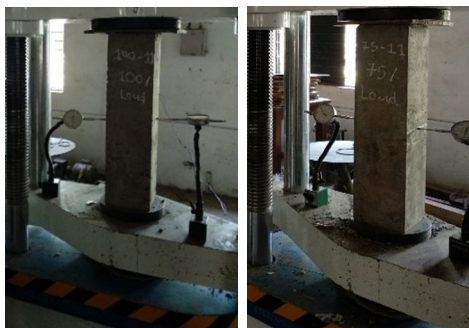
Fig. 3 testing of column specimen
