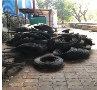
Fig 1: improper wire bundle staking
