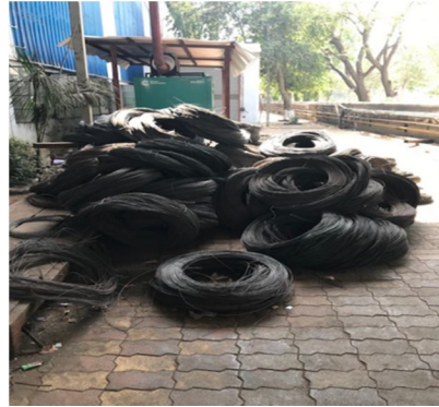
Fig 1: improper wire bundle staking
