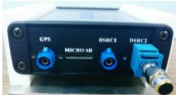
Figure 1: Input Side of After Safety Market Device
