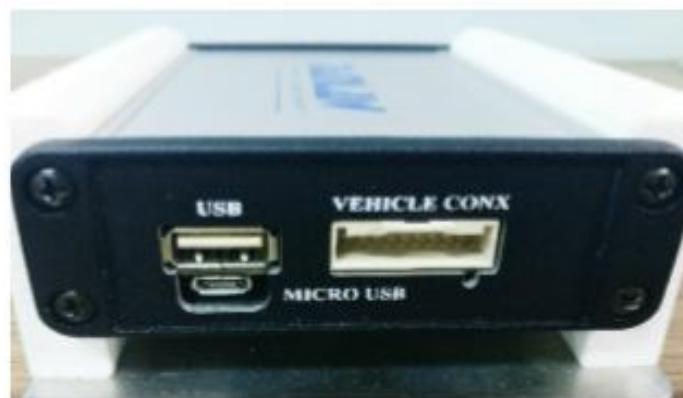
Figure 2: Output Side of After Safety Market Device
