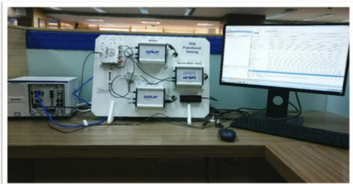
Figure 3: DANLAW HIL bench setup
