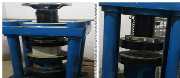
Fig. 2. Compression Test for Concrete Specimen and Mortar Specimen
