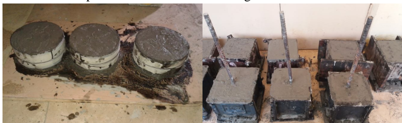
Fig. 4 Casting of Impact , Pullout and Cube specimen
