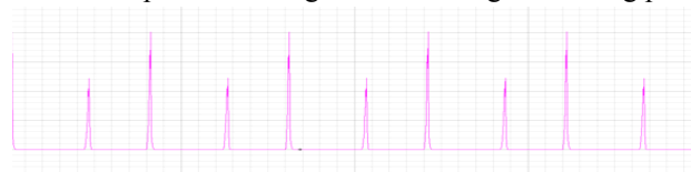
Fig.3(b) ) EP-DCO flip-flop power waveform in cadence tool.
