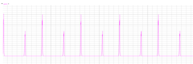
Fig.7(b) TSPC flip-flop power waveform in cadence tool.
