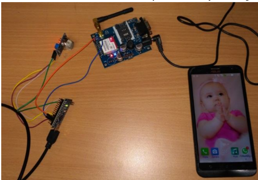
Fig.3.9 SMS Notification System
