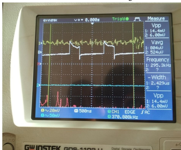
Fig. 12: PWM waveform with 1us + width
