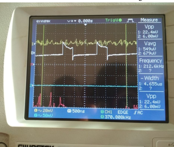
Fig. 13: PWM waveform with 2us + width
