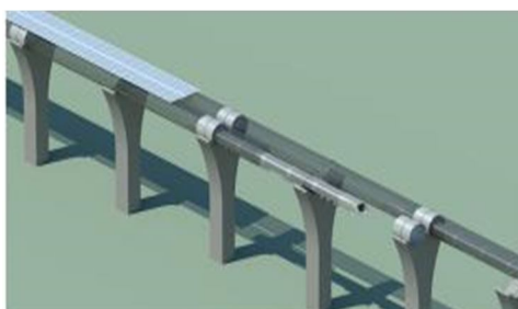
Figure : Hyperloop capsule in tube cutaway with attached solar arrays.
