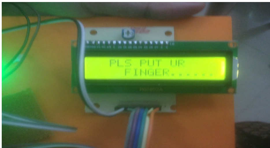
Figure 5.2.1 Screen shows that the LCD displaying to put finger on the Biometric scanner to capture the image.
