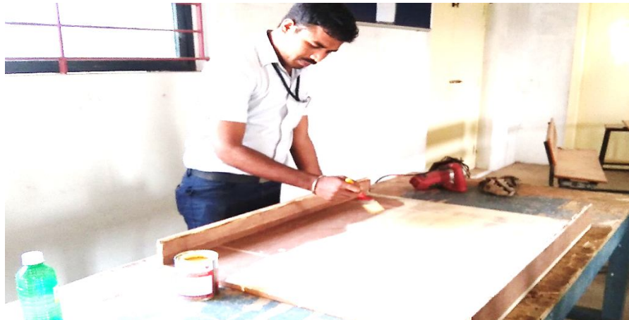
Fig. 2. 5: Painting wooden frame
