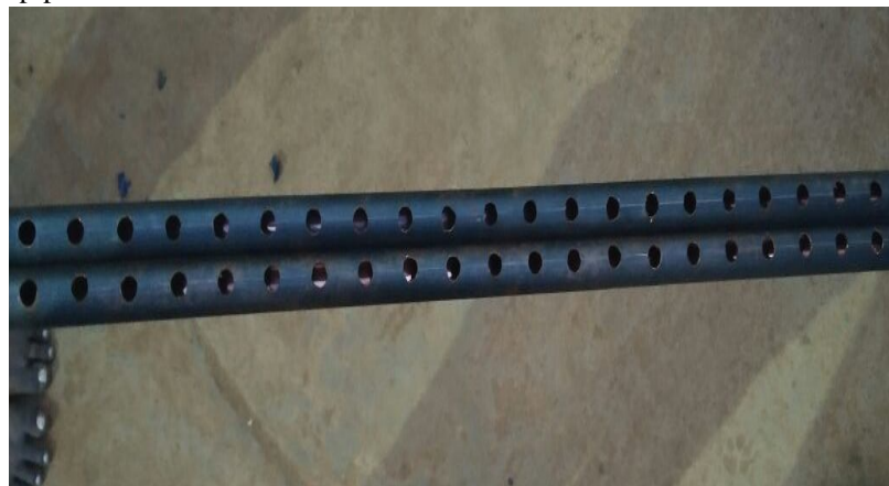
Fig. 2. 3: holed copper pipes
