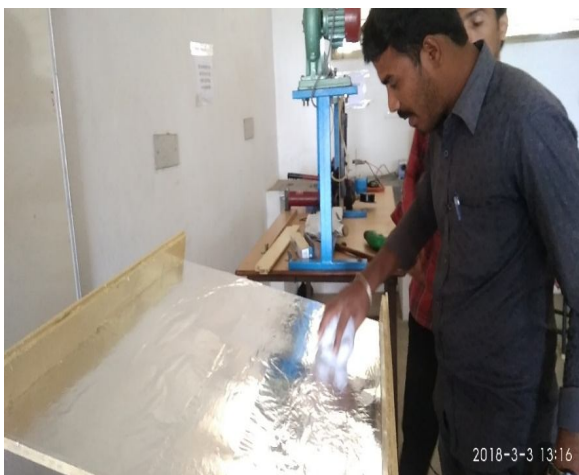
Fig. 2. 6: aluminium foiled frame
