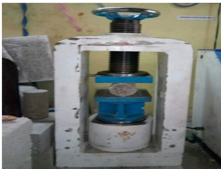
Fig 4a Tested specimen for split tensile
