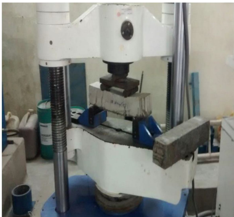
Fig 5a Tested specimen for Flexural strength
