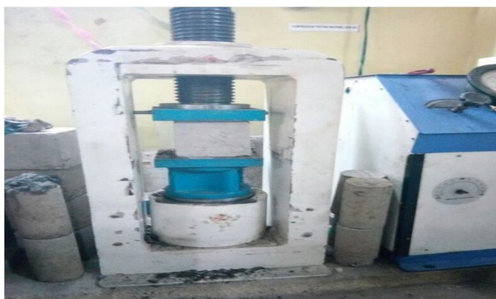
Fig 3a Tested specimen for compression
