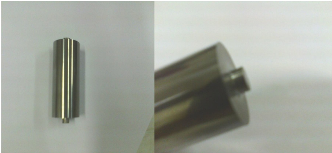
Figure 2.1 Tool with shoulder and pin.
