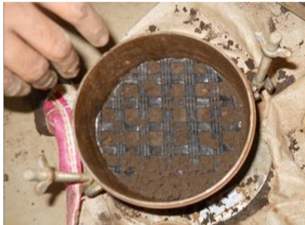
Fig:2 Geogrid material placed into CBR mould
