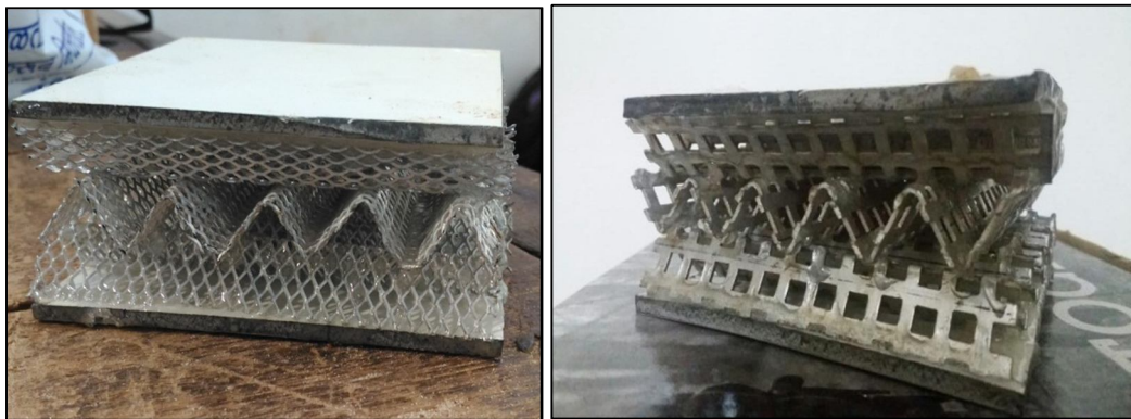
Figure 2.5 Samples of CWML Sandwich Panels
