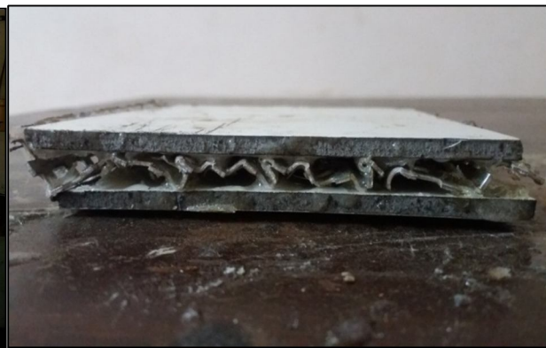
Figure 2.7 Compressed corrugated core sandwich panel
