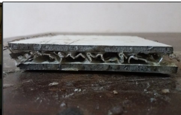
Figure 2.7 Compressed corrugated core sandwich panel
