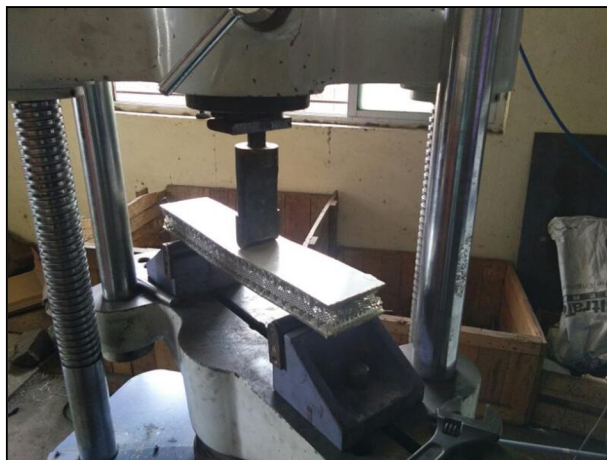
Figure 2.8 Bending Test Setup
