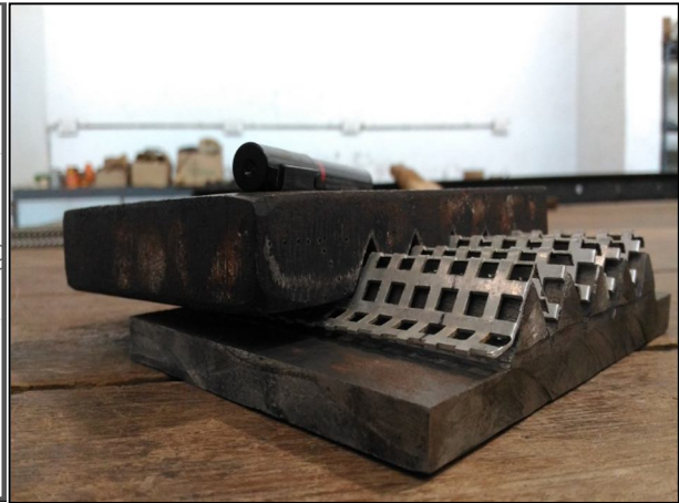
Figure 2.3 Manufactured die with corrugation angle of 55°
