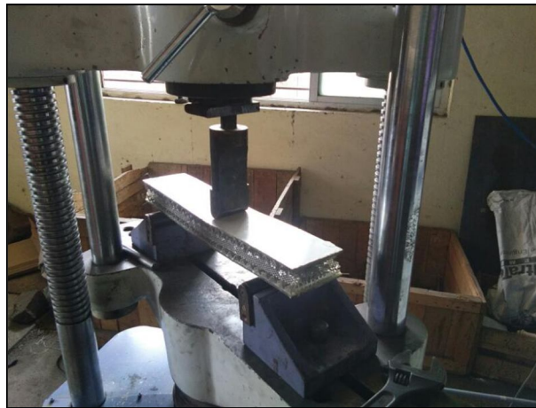
Figure 2.8 Bending Test Setup
