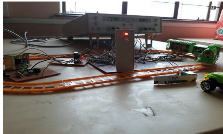
Fig.8. At arrival of the train, gate is closed
