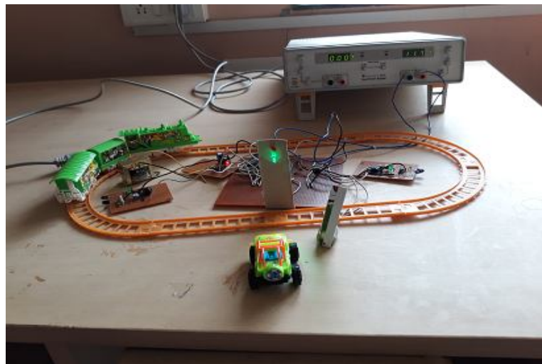
Fig.9. Gate is open after the departure of train
