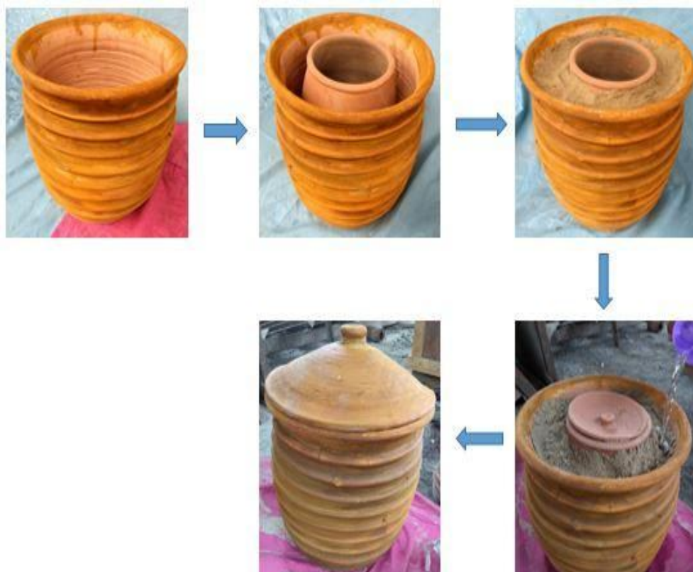
Fig.13: Assembly procedure (sand as filler)
