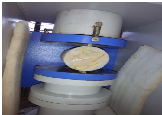
Fig 3: Split Tensile strength Test
