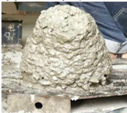
FIG 2: SLUMP TEST FOR FRESH CONCRETE
