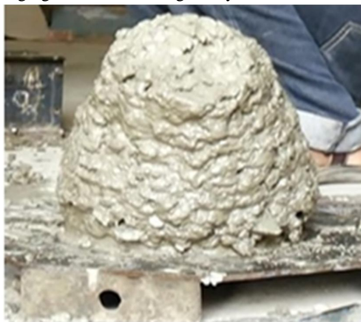
FIG 2: SLUMP TEST FOR FRESH CONCRETE
