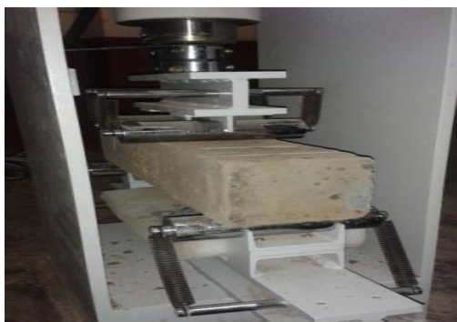
Fig 4: Flexural strength Test
