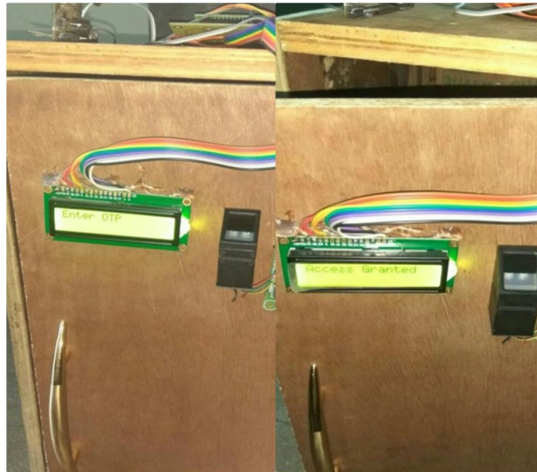
fig.(2) OTP Access
