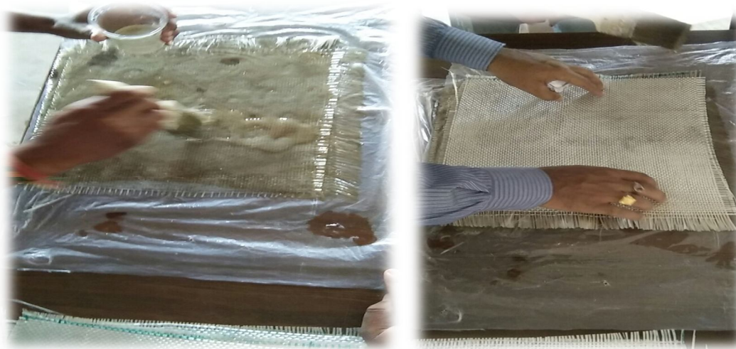
Fig11: Sample preparation by wet hand lay-up process
