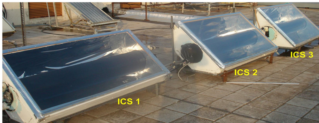
Fig. 17. Experimental ICS models mounted at the test field.[20]
