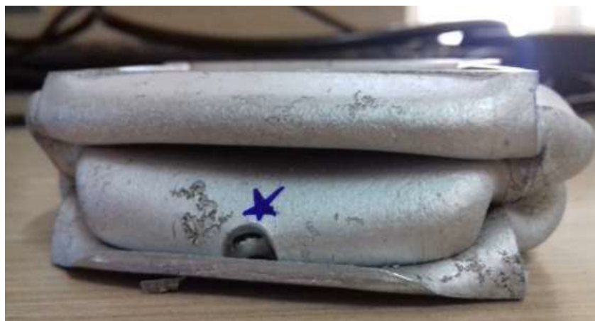
Fig. 25 Specimen After Complete Deformation (Test no. 4)
