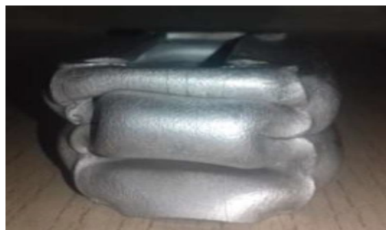
Fig. 19 Specimen After Complete Deformation (Test no. 1)
