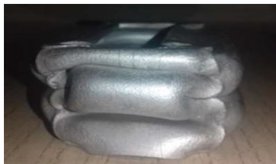
Fig. 19 Specimen After Complete Deformation (Test no. 1)
