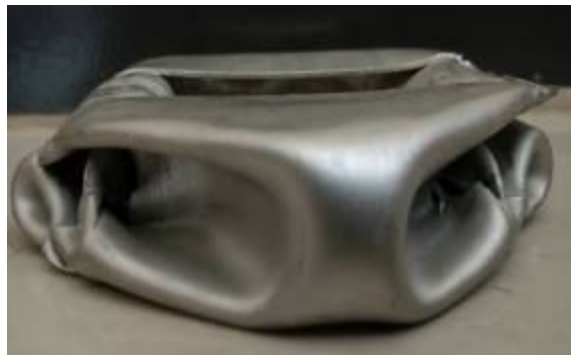
Fig. 21 Specimen After Complete Deformation (Test no. 2)
