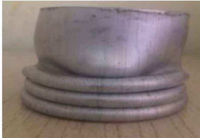
Fig. 23 Specimen After Complete Deformation (Test no. 3)
