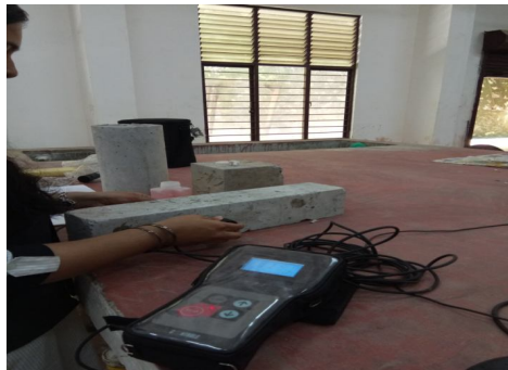
Figure 2: Ultrasonic pulse velocity test
