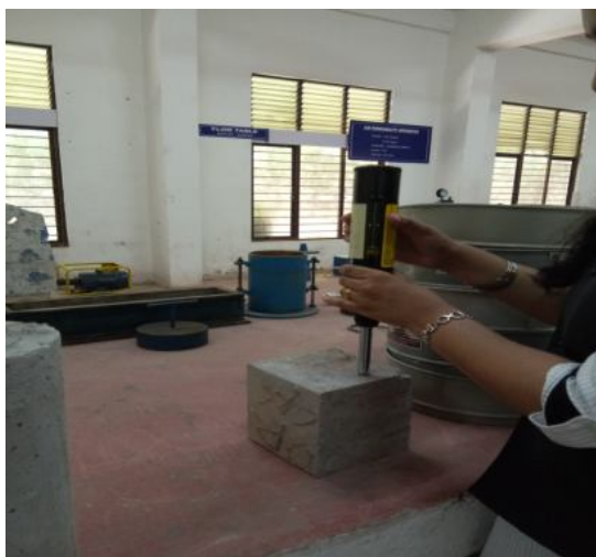
Figure 3: Rebound hammer test
