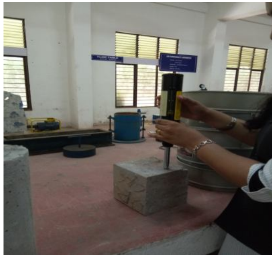
Figure 3: Rebound hammer test
