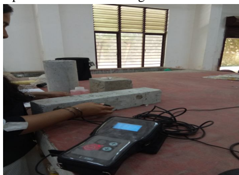
Figure 2: Ultrasonic pulse velocity test
